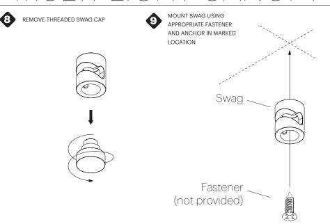
NOTE: Cable slot should face canopy center point.
